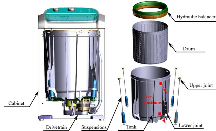
Figure 1: Illustration of a hang-suspension vertical axis washing machine. Fonte: [7].
