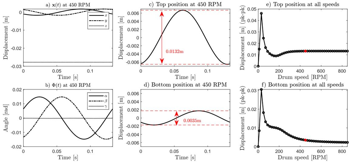
Figure 3: a) and b) represents the steady state response of the washer vibration. c) and d) are the radial displacements of the tank in the top and bottom position. e) and f) are the pk-pk top and bottom displacements of the tank for different spin speeds. Fonte:[7].
