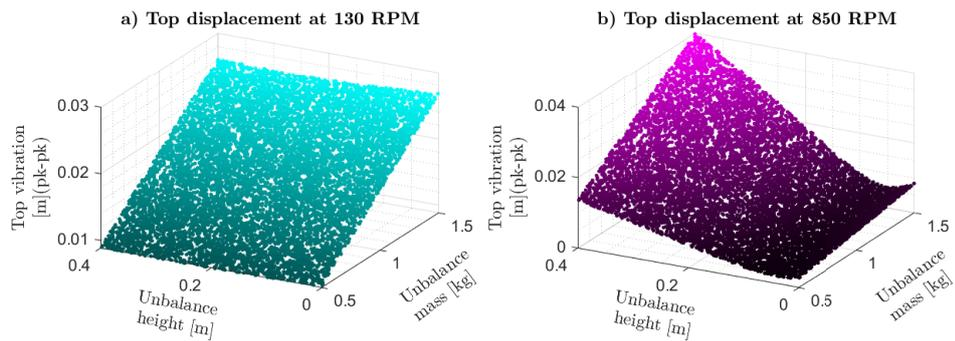
Figure 5: Scatter plot of the top displacement vibration amplitude (peak-to-peak) as function of the random variables samples. Fonte:[7].
