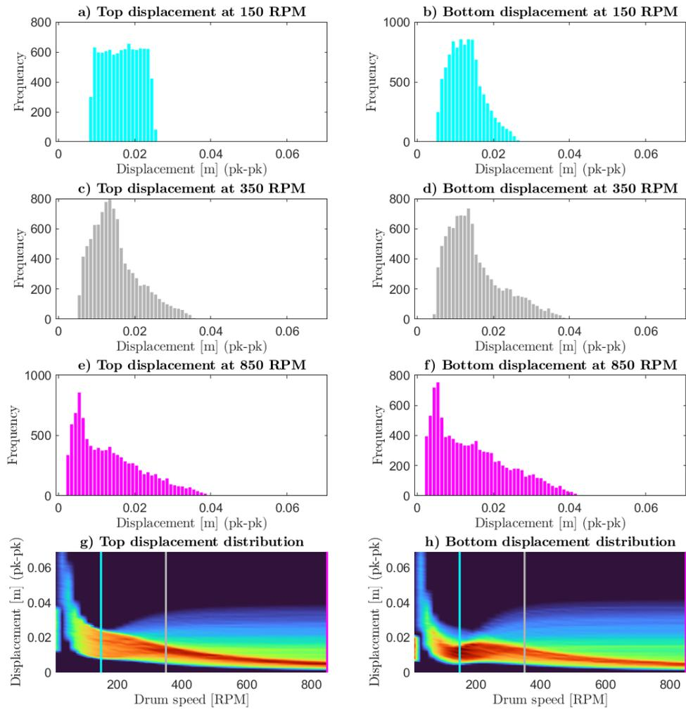
Figure 4: Probability distribution of the WG peak-to-peak vibration at different spin speeds. Fonte:[7].
