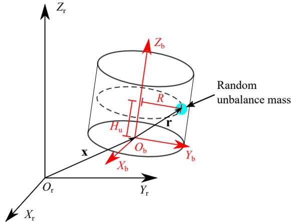
Figure 2: Schematic representation of the global and local frames. Characterization of the random unbalance through two random variables  $H_u$  and  $M_u$ . Fonte:[7].
